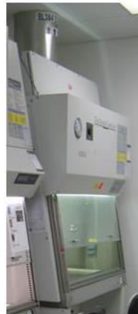
Fig. 7. MSC Class II Type 1 or B1 Front opening: A) sash, B) exhaust HEPA filter, C) supply HEPA filter, D) negative-pressure exhaust plenum
